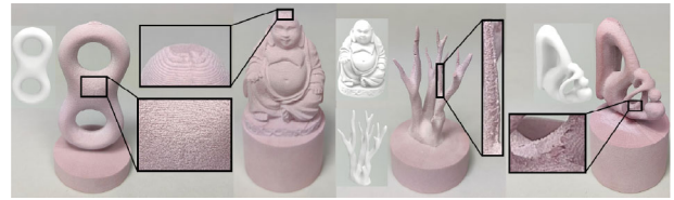
Figure 16: Fabricated results with detailed close-ups. This figure shows close-up photos of four fabrication results. They are Eight, Coral, Buddha and Fertility.
