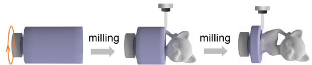
Figure 5: Demonstration of the fabrication process. After assembling the stock on the fixture, we mill the stock layer by layer along the rotation axis using the four-axis machine.
