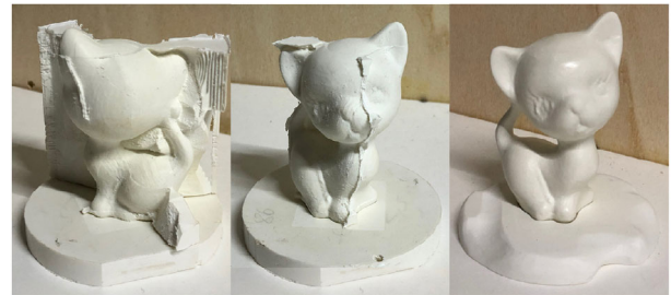
Figure 3: Manufacturing demonstration of the positional machining strategy. The figure is from Nuvoli et al. [NTM*21], which fabricates the Kitten model by carving it from a set of height-field patches and then applying manual post-processing work.
