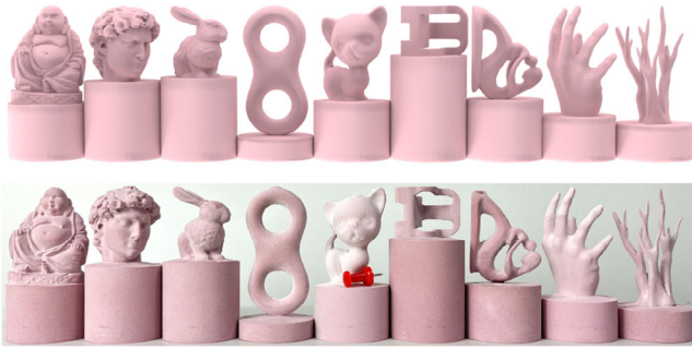
Figure 17: Fabrication results gallery. The upper portion of the figure displays a rendered view of the corresponding input 3D models. The lower portion showcases a collective image of the fabrication results.
