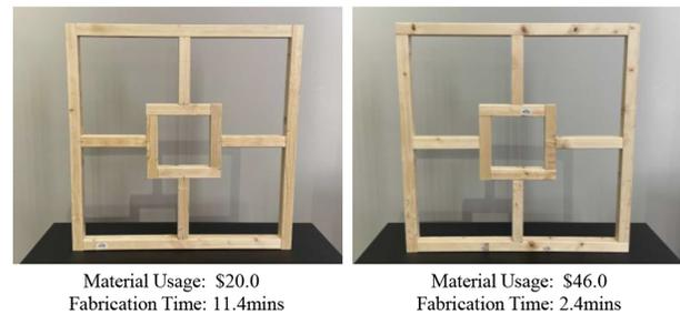
Fig. 11. Fabrication results of two window variations. The different designs and fabrication plans trade-off fabrication time and material usage.
